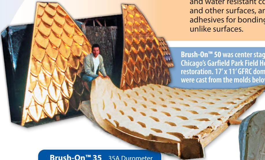
**Brush-On™ 50** was center stage during Chicago's Garfield Park Field House restoration. 17' x 11' GFRC dome panels were cast from the molds below.
