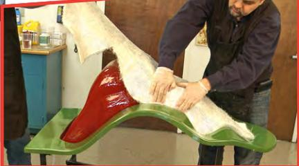
2. The cured bag is removed. Resin gel coat and glass are applied to the tool.
