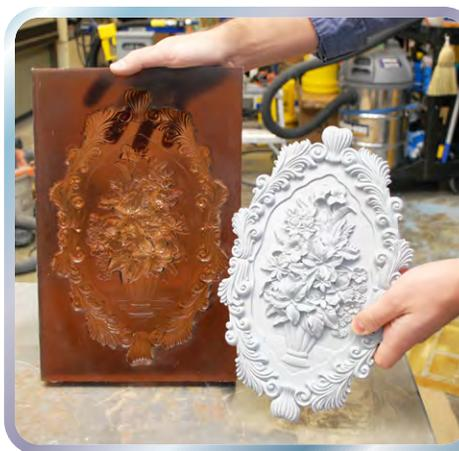
PMC™-746 molds are used for casting heavily filled polyester furniture elements at Union City Mirror in New Jersey.
