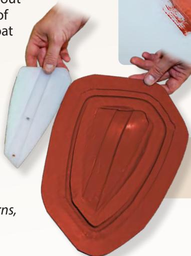
Ultratough **EpoxAcoat™ RED** tool is ready to make composite parts for motorcycles.
