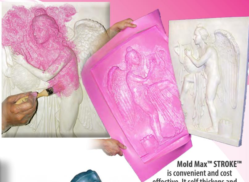
**Mold Max™ STROKE™** is convenient and cost effective. It self thickens and holds a vertical surface for making detailed brush-on molds.
