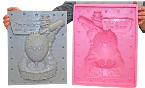
**EpoxAcast™ 655** is commonly used for vacuum forming dies.
