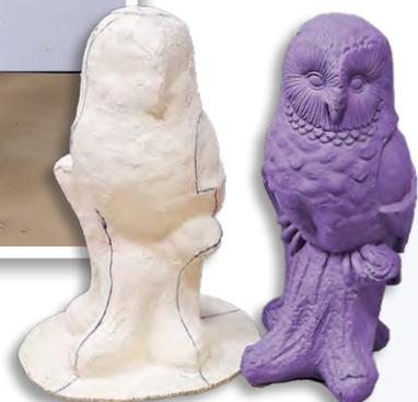
The HX-974™ mold is used to make a casting.
