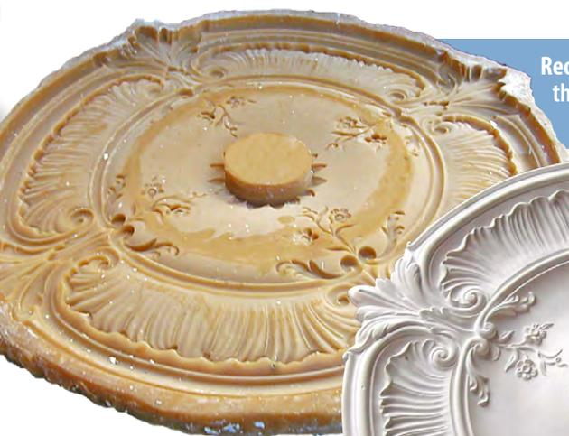
ReoFlex™ mold rubber picks up all the intricate detail from this wall plaque and ceiling medallion.
