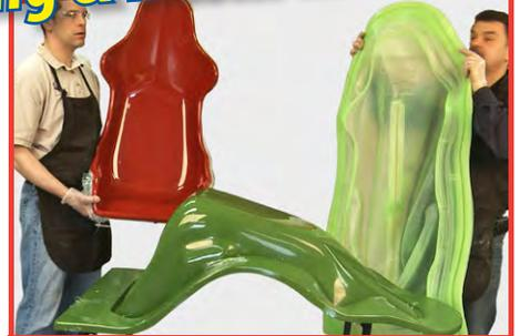
4. The cured composite car seat is removed and ready for installation.
