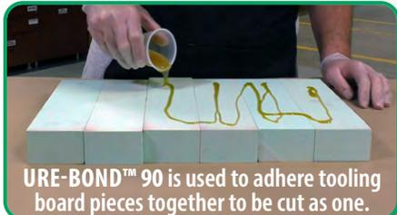
URE-BOND™ 90 is used to adhere tooling board pieces together to be cut as one.
