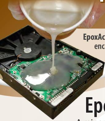
EpoxAcast™ 650 is used for encapsulating sensitive electronics.
