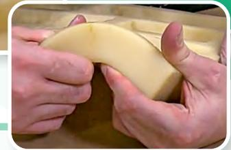
Ure-BOND™ II is being used to repair a tear in a urethane mold.
