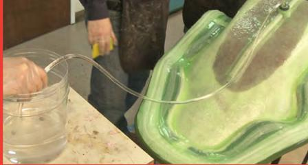
3. The bag is repositioned and resin is drawn in, saturating the glass.
