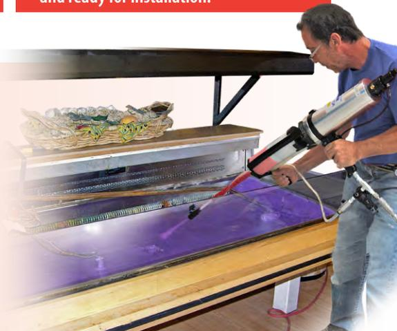
Silicone liners made with EZ~Spray™ 35 for repairing hundreds of grocery store refrigeration units.
