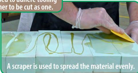
A scraper is used to spread the material evenly.
