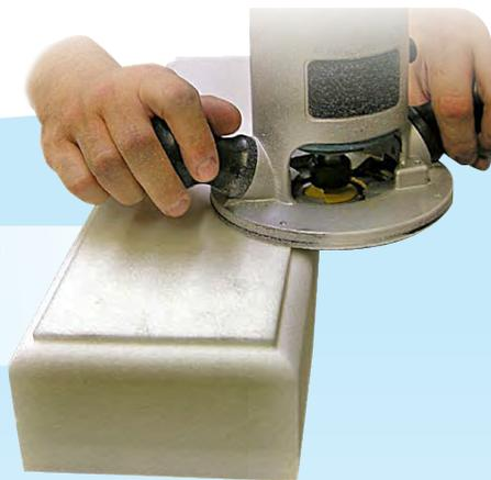
Cast custom block of FOAM-iT!™ 8 is used as a machinable modeling board.
