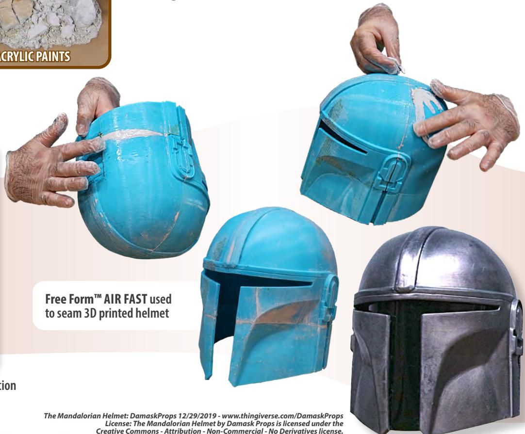
Free Form™ AIR FAST used to seam 3D printed helmet
