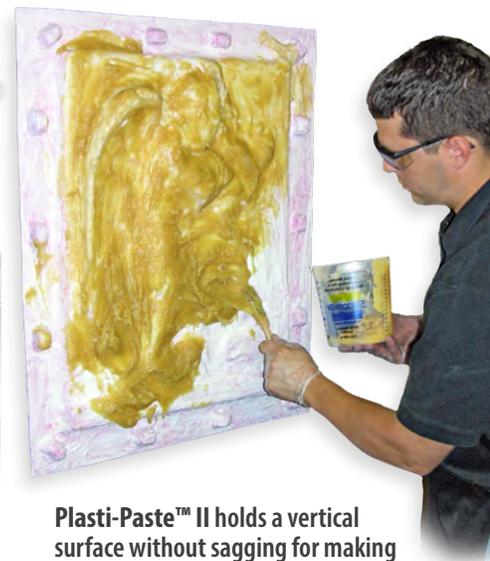
**Plasti-Paste™ II** holds a vertical surface without sagging for making lightweight mother molds.
